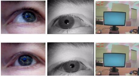
Figure 2. Examples of recorded eye images. The images to the left are from the webcam. The grey images in the center and the images to the right are from the Dikablis eye and field camera, respectively. The red point on the screen shows the point of gaze.
