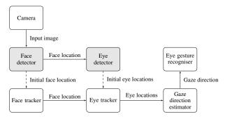
Figure 2: Architecture and information flow within the eye gesture recognition system. Grey rectangles indicate processing components that are only called during initialization.
