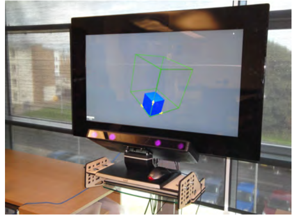
Figure 2: The Microsoft Pixelsense mounted vertically and the Tobii X300 eye tracker placed on a custom laser cut wooden shelf.
