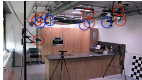
Fig. 6: Kitchen environment used for recording our dataset. The kitchen was fully functional and instrumented with ceiling-mounted cameras (red circles) and microphones (blue circles).
